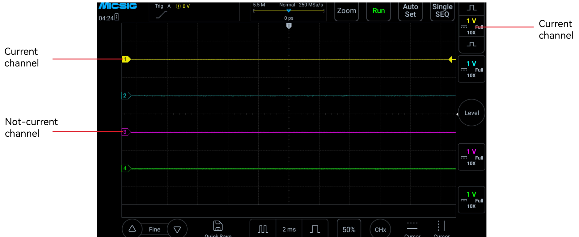
Figure 5-2 Current Channel and Non-Current Channel
