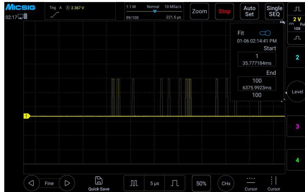
Figure 12-13 Segmented storage fitting view
